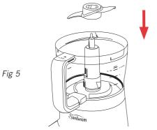
**Warning:** Use caution, as blades are sharp. Always handle the processing blade by its central plastic section.
